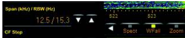
Figure 3: The levels of the markers shows resolution bandwidth (RBW), which is displayed in Hertz in a window on the left of Perseus.
