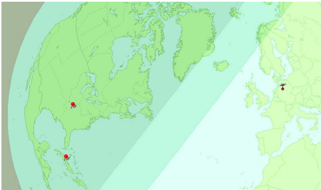
Figure 20: Shows the position of the grayline on December 30th at 1000 UTC, globe projection. Nashville and Habana are shown by pushpin icons, and the receiver location is indicated by a Yagi antenna icon.
