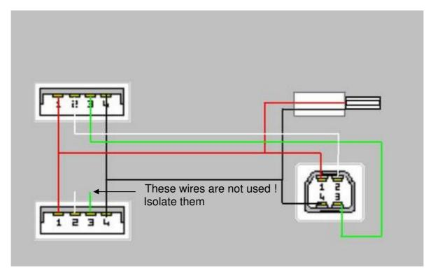
Wire colour code is correct for most usb cables but some brands use different colours. Make sure to measure them before use!
