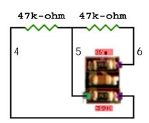
•The finished mod should look similar to the picture below. Note the color-coding used to easily identify the center (yellow & green) and end (blue pair & white pair) connections.
