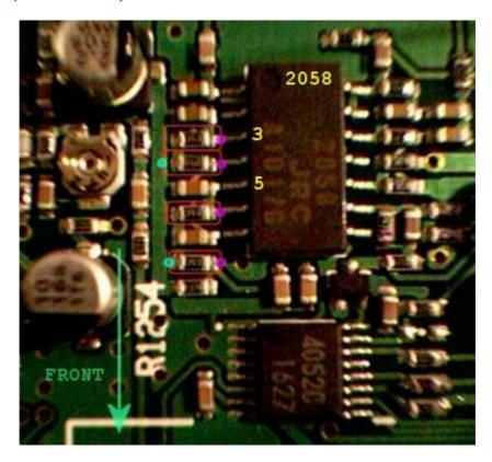
•These schematics show the six connections from the four 47k-ohm resistors (green below). Wires 2 & 5 make up the 'center' connections, whereas, wires 1 & 3 and 4 & 6 make up the 'end' pairs.
