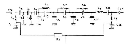
Component list: C1, C11, C12 = 0.01 uFC13 = 220 pFC3 = 4700 pFC2, C4 = 8200 pFC5 = 2200 pFC6 = 3300 pFC7 = 820 pFC8, C10 = 1800 pFC9 = 680 pFL1, L8 = 470  $\mu$ H L3, L5 = 4,7 uHL2 = 10 uHL4, L7 = 6,8 uHL6 = 3,3 uHR1 = 100 ohm
