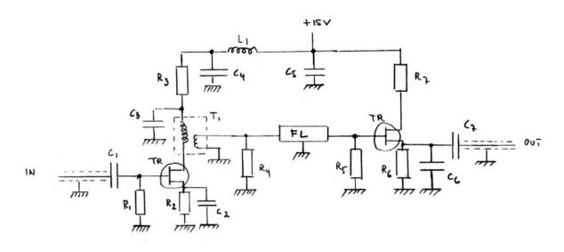
Components: C1, C2, C3, C4, C5, C6, C7 = 0,01 uF R1 = 10K R2, R6 = 470 R4, R5 = 2,2K R3 = 100 R7 = c:a 19K ( try out the value to get the same gain as without the new filter unit) L1 = 0,33 mH T1 = 455 kHz 20K:5K transformer (TOKO or similar) TR = MPF102 or similar FL = CFK455H or CFK455I
