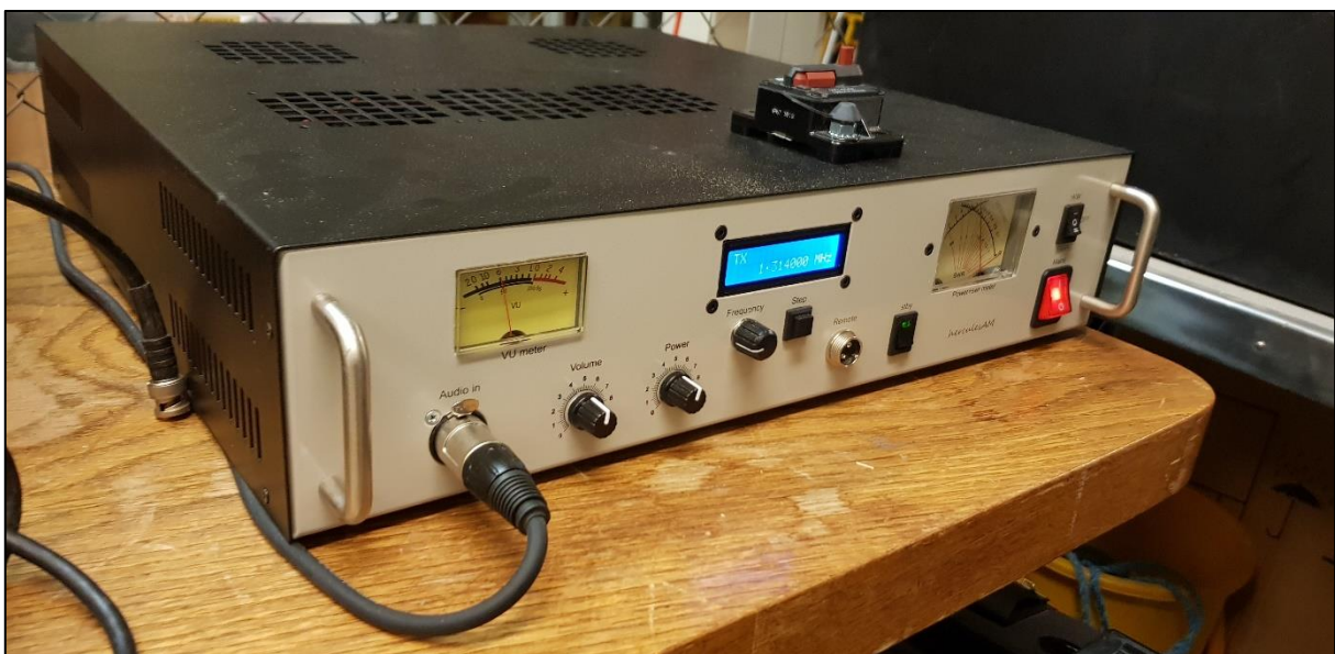
1kW Hercules transmitter of which 700 watts is regularly used. (Foreningen Bergen Kringkaster, picture: Northern Star Media Services AS)
