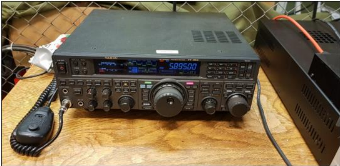
Converted Yaesu FT-950 100 watts transceiver delivering 30-35 watts on 5895 in AM mode.
