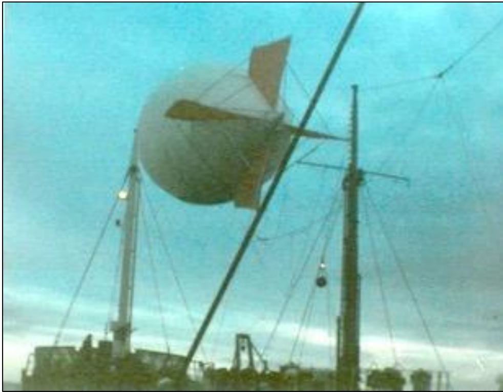
Laser 730 729 kHz second test with 50 kW on Saturday, January 28th, 1984 with balloon aerial from the ex Norwegian ship "Tananger" then "Communicator" in early 1984. The same type of antenna had already been used on the VOA Ship "Courier" off the Dodecanese Islands in the 50s. (Jelle Boonstra archive)
