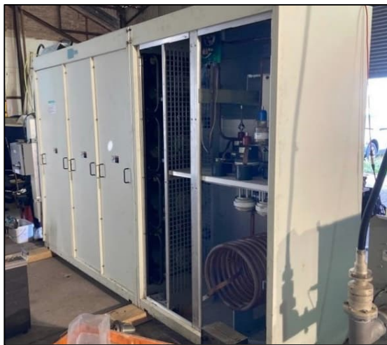
Figure 1 and 2: Two views of our new transmitter part way through its rebuild. (Pictures:Ray Clark)
