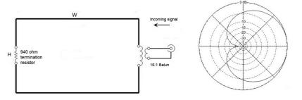
The baluns for both antennas are wound on the same type of toroids and with the same number of turns. FT114-43 toroids are recommended.
