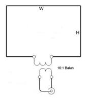
The ALA100 broadband loop is a bi-directional antenna and has an elliptical reception pattern.
