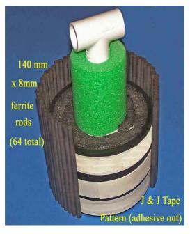
6) Stand the inner core and rubber plumbing coupler assembly vertically on the flush end, as shown at left. Remove the metal hose clamps from the rubber plumbing coupler, if not done previously. To fill up the slight horizontal slots left on the plumbing coupler after removal of the hose clamps, some ½" J & J tape or a folded length of 1" tape (adhesive side out) may be used until the slots are level with the main rubber surface of the plumbing coupler.
