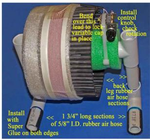
on slippery or wet surfaces. This completes construction of the 7" FSL antenna.
